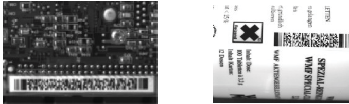
Figure 3: The PDF 417 code for electronic component (left) and hazardous materials (right) labeling
