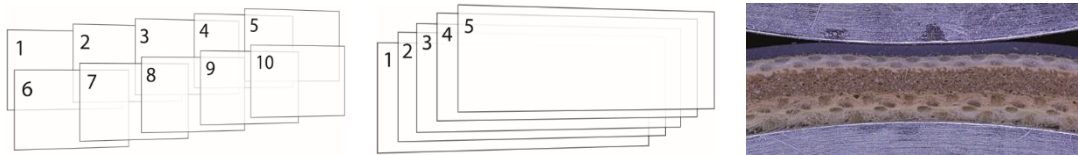
Figure 10: Acquisition and preparation of multiple microscopic images in order to get one supersized image a) stitching of ten images b) stacking of five stitched images c) one well-focused result image in high-resolution
