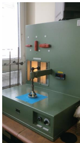
Figure 1. Air permeability measuring device
