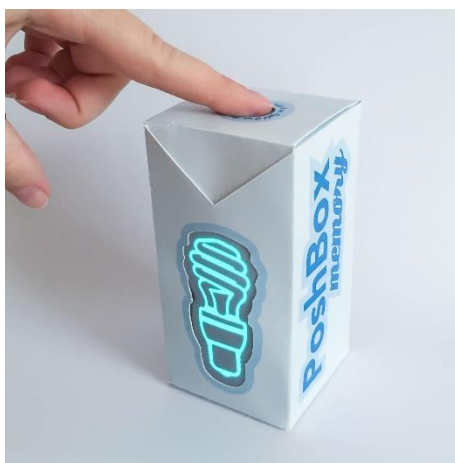
Figure 4: Interactive packaging with touch sensitive sensor and EL screen
