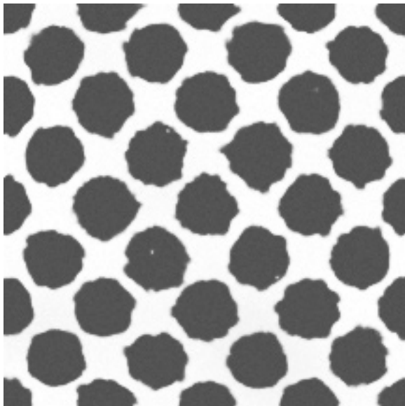
Picture 2: Halftone dots, that are printed with conventional offset technology. [4]
