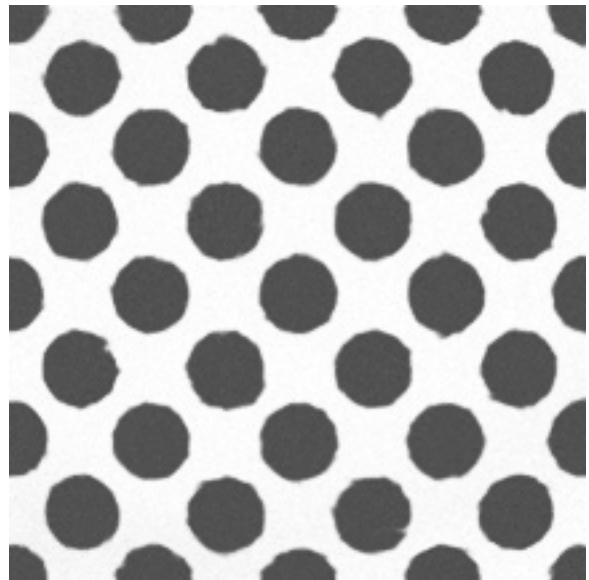
Picture 3: Halftone dots, that are printed with waterless offset technology. [4]
