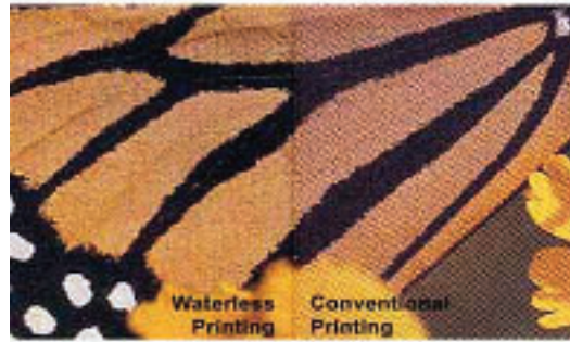
Figure 2. waterless image vs. conventional offset image (comparison based on differences in resolution)
