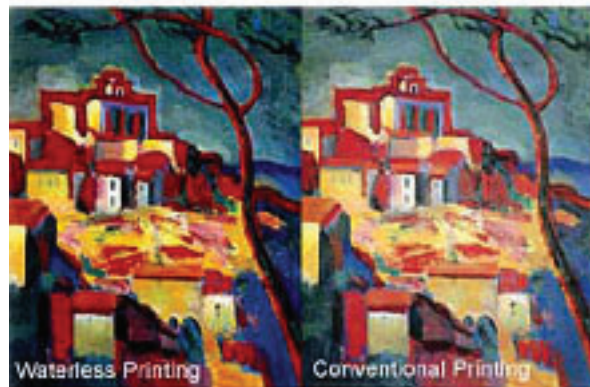
Figure 3. waterless image vs. conventional offset image (comparison based on possibility to reproduce tiny details)
