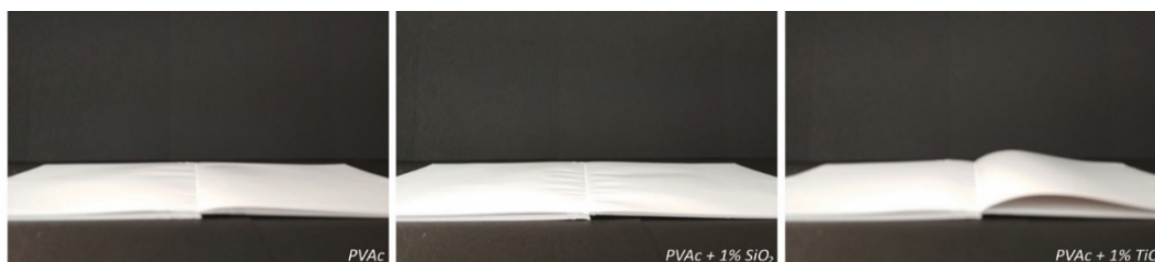
Figure 2: Opening behaviour of WFC book blocks (PVAc; PVAc + 1%SiO 2 ; PVAc + 1%TiO 2 )
