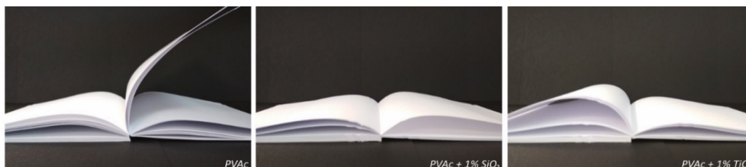
Figure 1: Opening behaviour of WFU book blocks (PVAc; PVAc + 1%SiO 2 ; PVAc + 1%TiO 2 )
