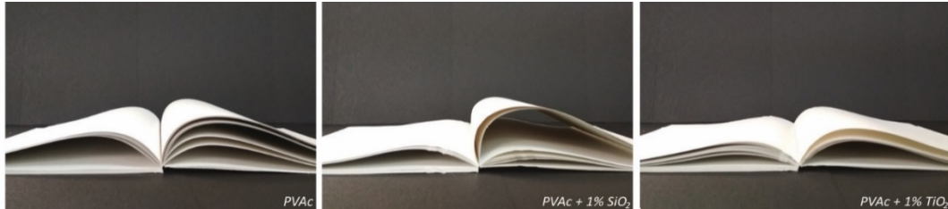
Figure 5: Opening behaviour of CR office book blocks (PVAc; PVAc + 1%SiO 2 ; PVAc + 1%TiO 2 )
