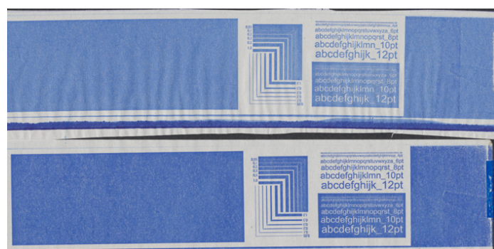
Figure 3: Print samples of the base paper (upper no plasma treatment lower after plasma treatment)
