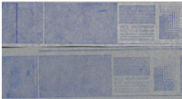
Figure 4: Print samples of the waxed paper (upper sample wax 2 lower sampler wax 1 sample before plasma treatment)
