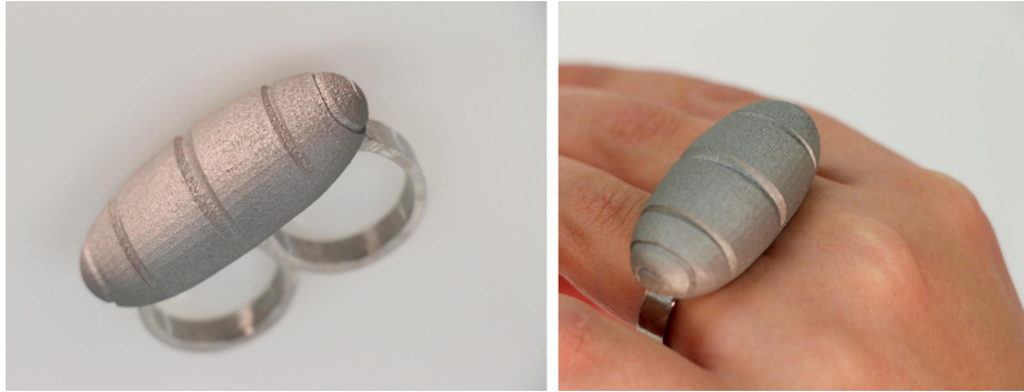
Figure 11: Ring printed with SLM technology, author: Tina Dovjak
