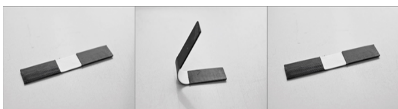
Figure 3: Shape recovery cycle of printed primitive; Phase 1 (left) – printed flat structure, Phase 2 (center) - self-transformation in hot water, Phase 3 (right) - transformation with force and hot water back into flat structure.
