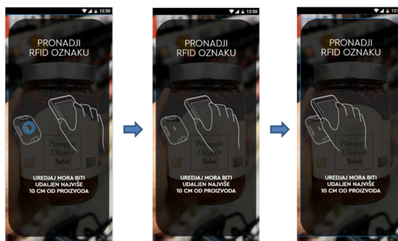
Figure 3 Finding correct distance between the phone and the indicator
