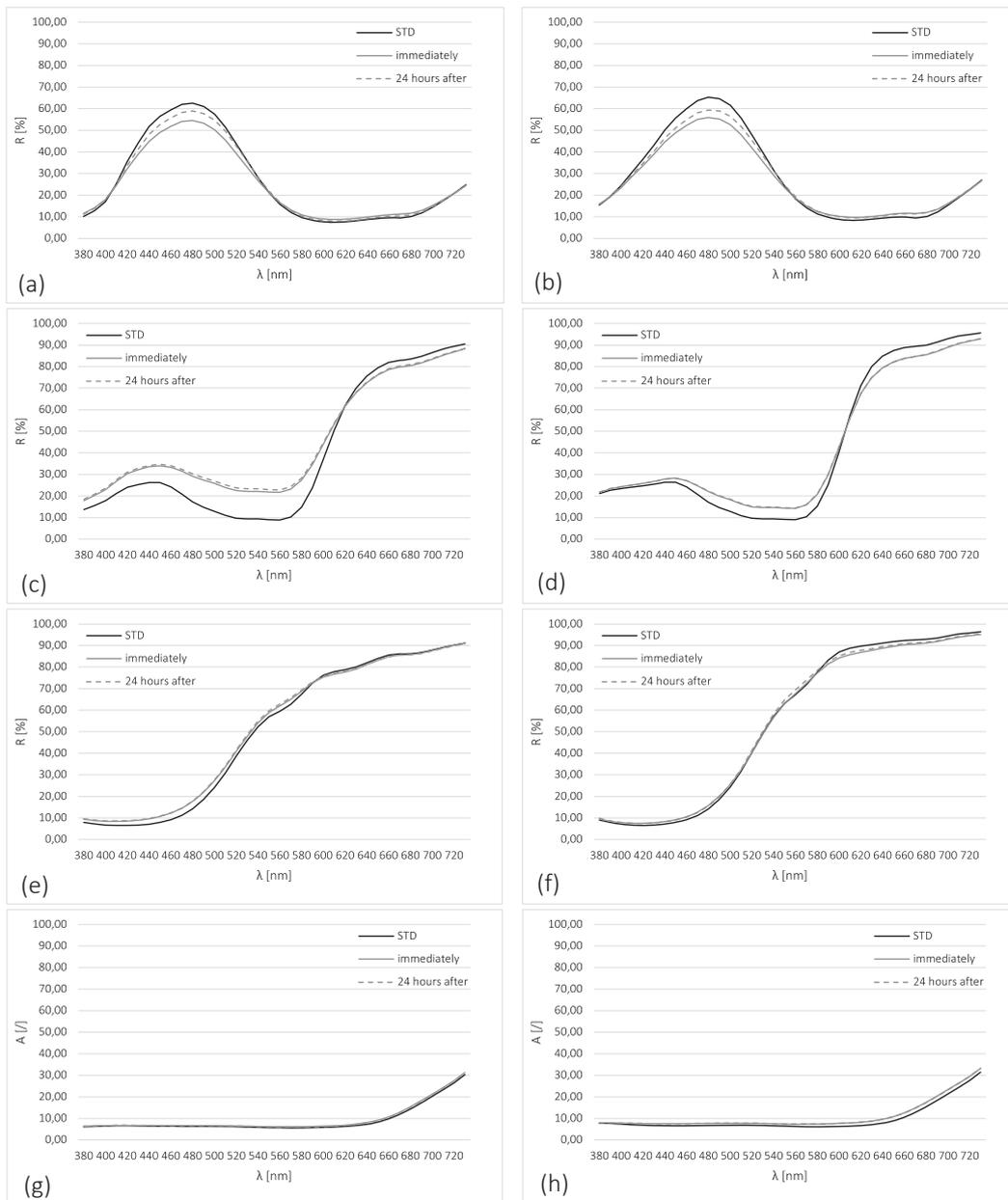
Figure 5: Reflection spectra of cyan (a, b), magenta (c, d), yellow (e, f) and black (g, h) prints on office paper PPO (left column) and permanent paper TPI (right column) before (STD), immediately and 24 hours of exposure to the high-pressure mercury lamp
