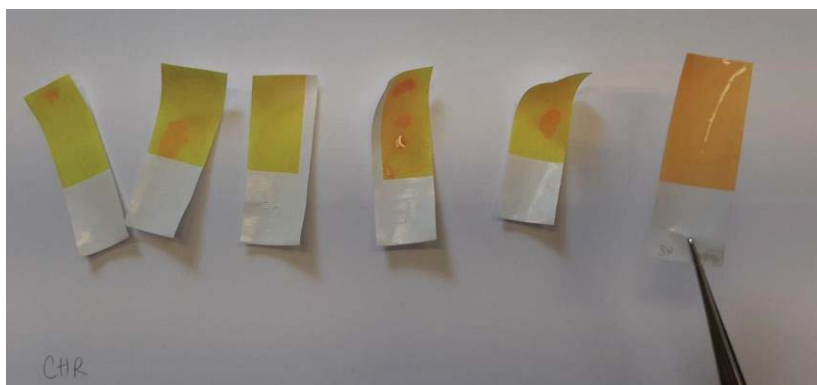
Figure 5: Change in the colour of the print as a result of the ethanol endothermic evaporation reaction on the CHR sample at room temperature ( 23\pm 2^{\circ}\text{C} ) indicating a temperature below 12^{\circ}\text{C} in areas where coloured in orange
