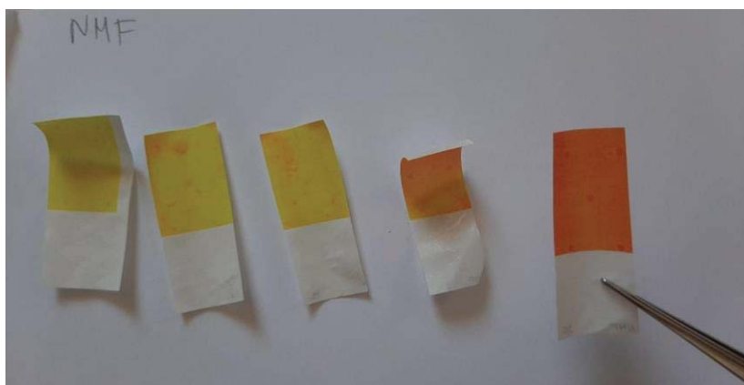
Figure 6: Change in the colour of the print as a result of the ethanol endothermic evaporation reaction on the NMF sample at room temperature ( 23\pm 2^{\circ}\text{C} ) indicating a temperature below 12^{\circ}\text{C} in areas where coloured in orange
