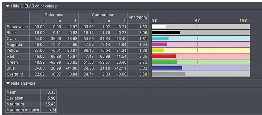
(b) CIE report and analysis color difference (e) of ECE 6 (0/-5) Figure 6: Display the total color difference ( \Delta E^*_{00} ) from Prinect Color Toolbox 12.0
