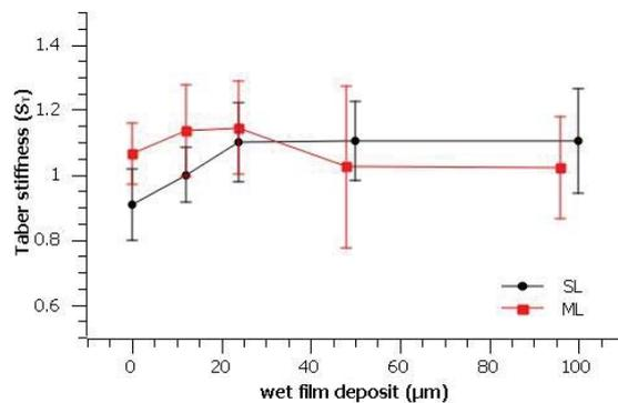
Figure 5: Taber stiffness of samples in relation to wet film deposit thickness
