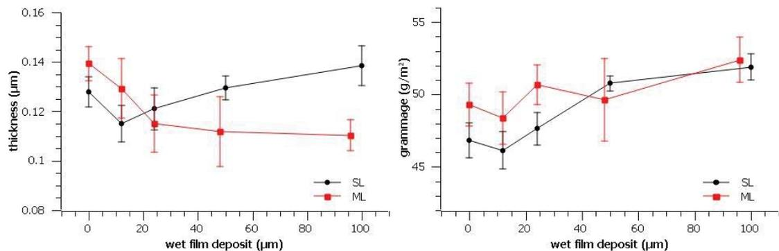
Figure 1: Changes in thickness (left) and grammage (right) of the samples in relation to wet film deposit thickness
