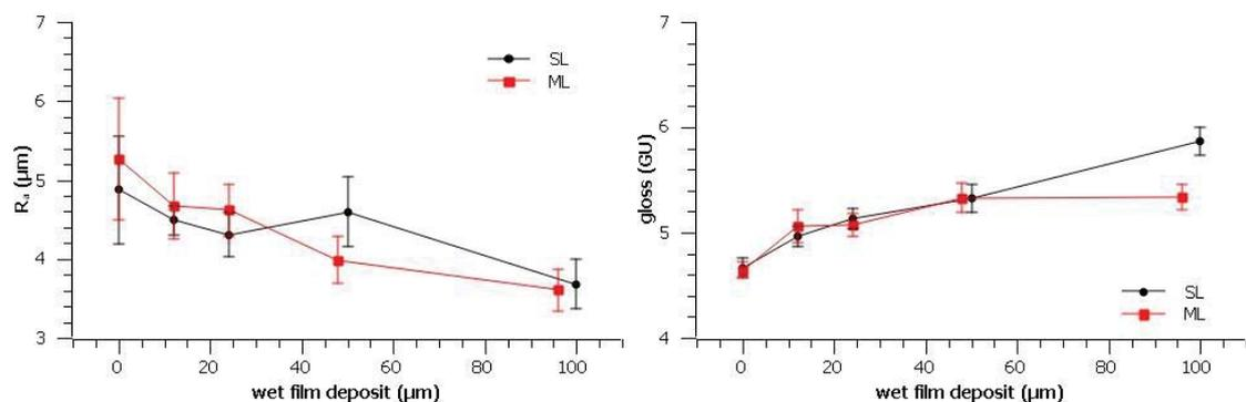
Figure 2: Average roughness  $R_a$  (left) and paper gloss (right) in relation to wet film deposit thickness
