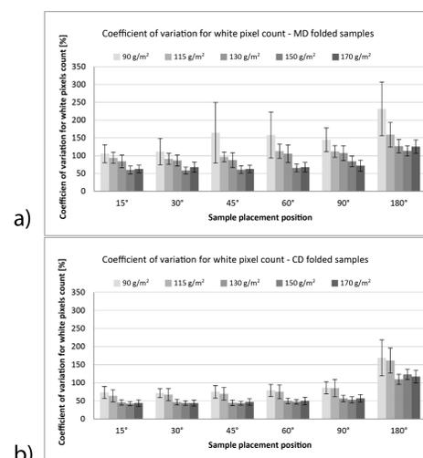
Figure 2 Coefficient of variation for white pixel count of samples folded in machine (a) and cross direction (b)
