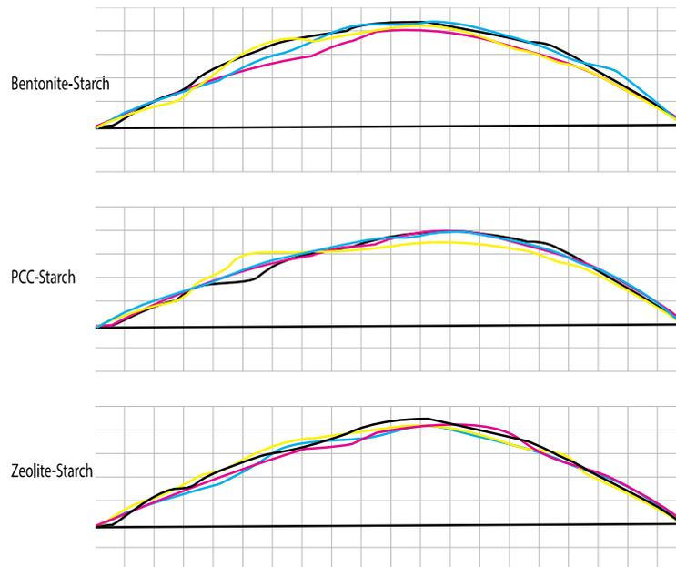
Figure 2: PCC-starch, bentonite-starch and zeolite-starch coatings dot gain curves
