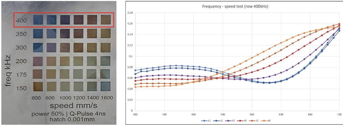
Figure 6: Frequency-speed test results at 400 kHz
