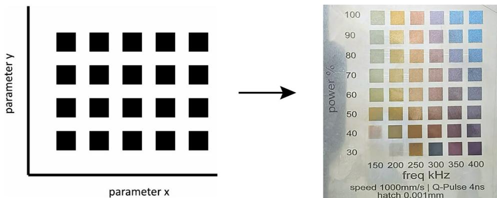
Figure 1: Laser parameter matrix for color testing
