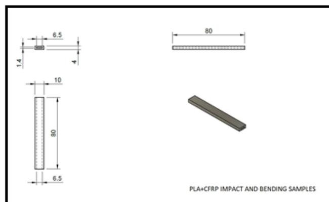
Figure 4: Technical drawing of the impact and bending test specimens
