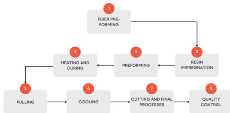
Figure 1: CFRP plate production method flow chart
