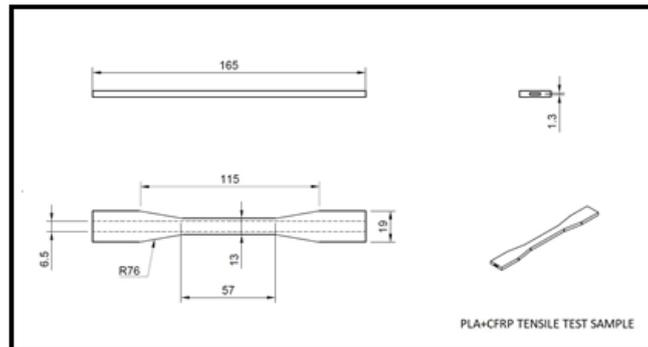
Figure 3: Technical drawing of the tensile specimens
