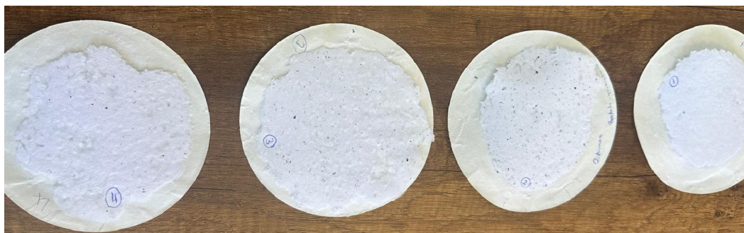
Figure 5: Papers produced using chemical process and enzymatic process (Enzyme treated deinking printed paper (EDPP), chemical deinking printed paper (DPP), Defibrillated undeinking printed paper (UPP), deinking base paper (DBP) respectively)
