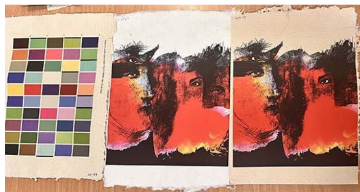
Figure 9: Fine art printing and profile process on Hemp + Seaweed coated paper
