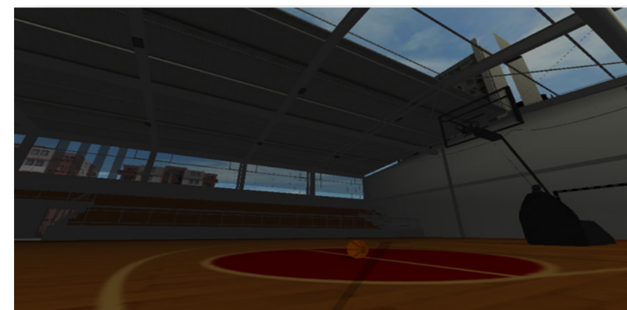
Figure 3: Simulation of the illumination in the interior of the sport hall in daylight, modulated when passing through the electrochromatic film in a shaded state. The film's transmission coefficient main value is 57.06%. The solar range AM 1.5 is fallen light and the interior lighting is switch off
