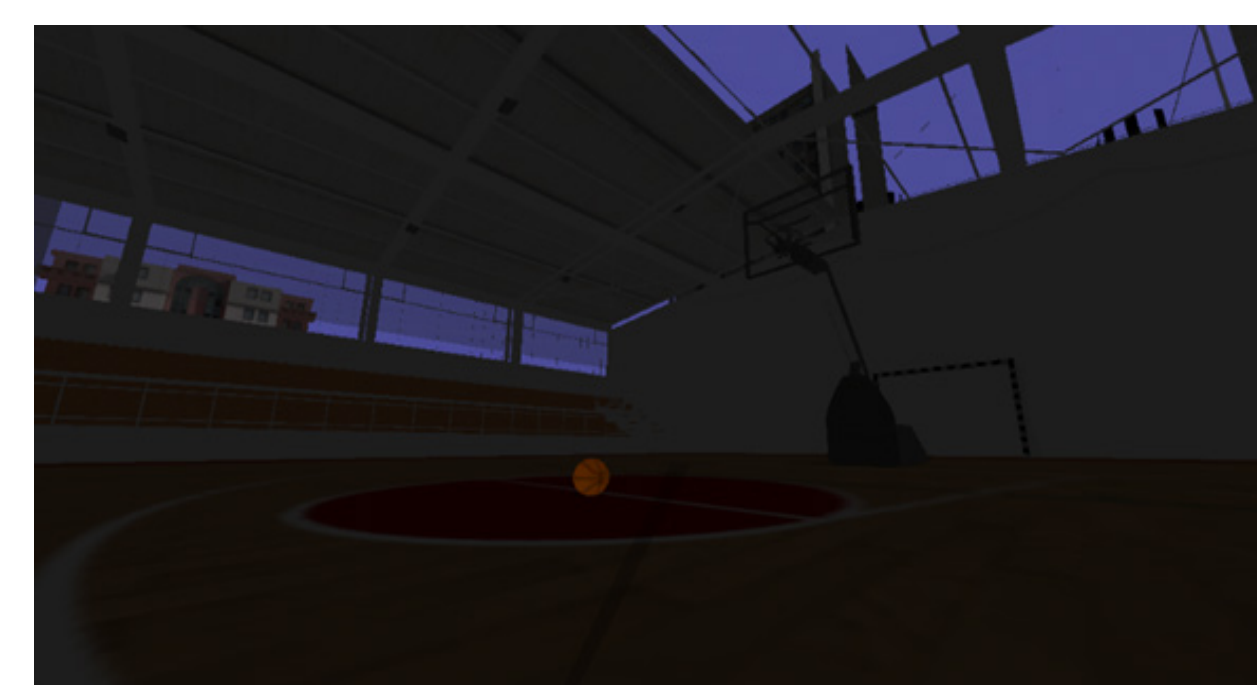
Figure 4: Simulation of the illumination in the interior of the sport hall in daylight, modulated when passing through the electrochromatic film in a colored state. The film's transmission coefficient main value is 20.0%. The solar range AM 1.5 is fallen light and the interior lighting is switch off
