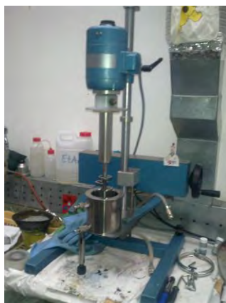
Figure 2: VMA-GETZMANN GMBH D-51580 Reichshof type bead mill
